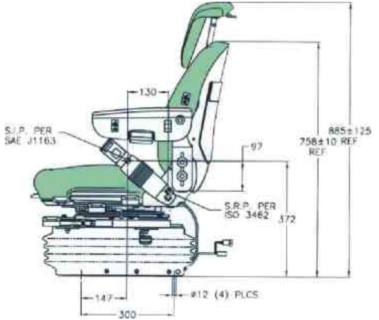
Large very low frequency, VRS Computer Controlled, plug & play Active-S air suspension, with three position ride selector & Airide® high volume air spring.
